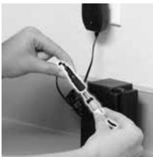
**Step 2:** Take the gray cord that is connected to your battery and plug it into the battery charger cord. While the battery is charging, the light on the charger will be solid red.
